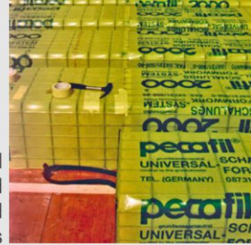
Formwork material for ribbed slabs and panelled slabs
